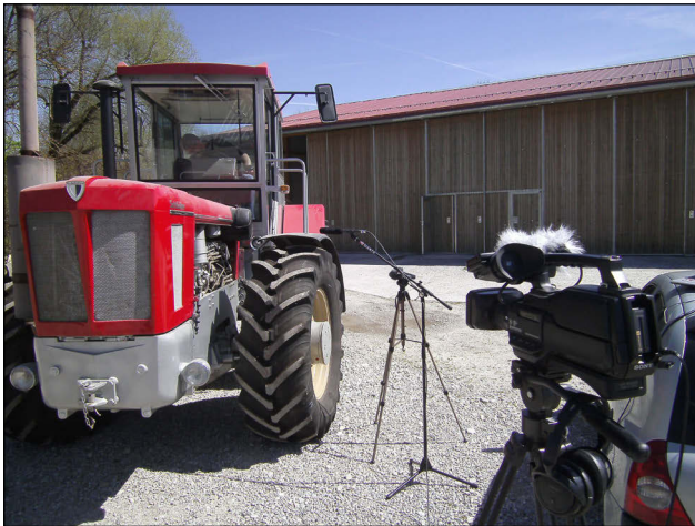
Figure 10-1: Recording the sound of a tractor on-site.
